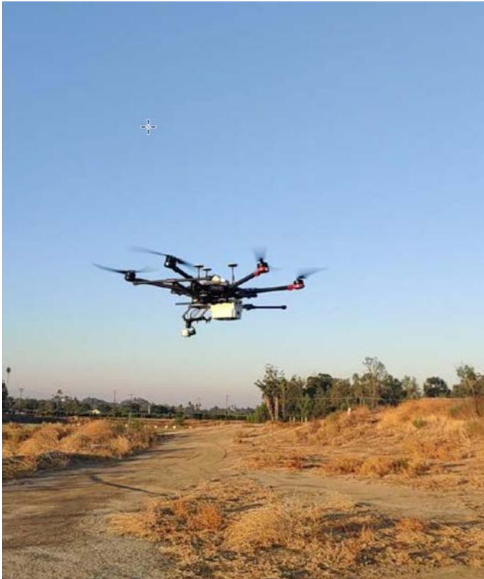
Don Collins' group uses drones to measure ozone and other pollutants
