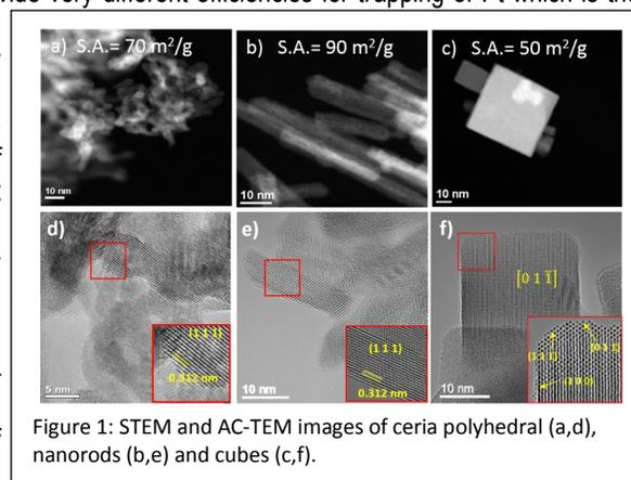
Figure 1: STEM and AC-TEM images of ceria polyhedral (a,d), nanorods (b,e) and cubes (c,f).
