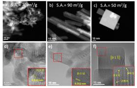
Figure 1: STEM and AC-TEM images of ceria polyhedral (a,d), nanorods (b,e) and cubes (c,f).
